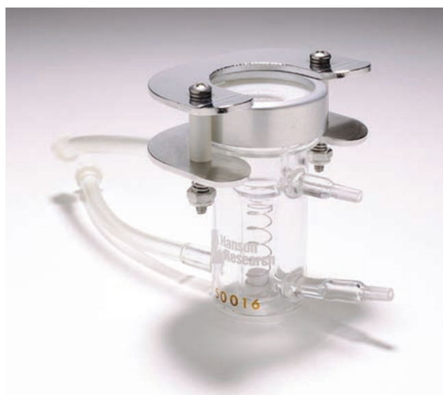
Figure 1. Vertical diffusion cell (VDC) assembly.
